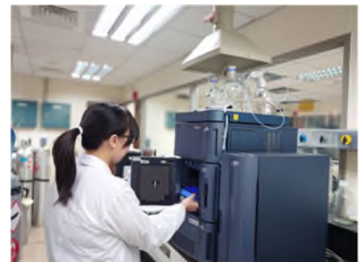
絕緣油中糠醛分析 Furanic Compound Analysis of Transformer Oil
