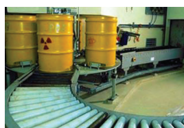
▶ 低放射性廢棄物固化裝桶情形 Flasking solid low-radioactivity waste
