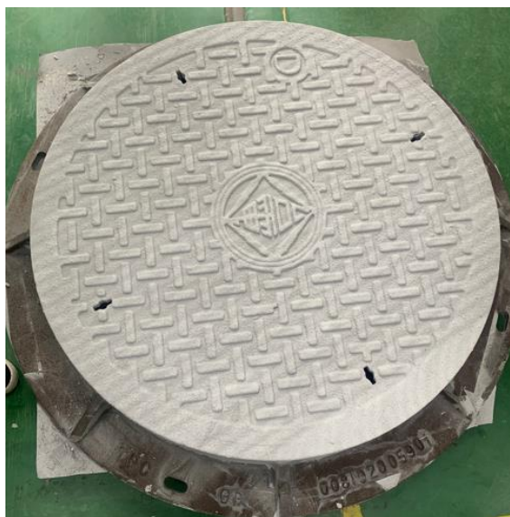
Figure 1. The photo shows a manhole cover with the anti-skid coating developed by TPRI.
