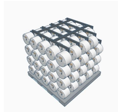
Figure 2. Demonstration of the Rack Fixture for 99 Single-Phase Smart Meters
