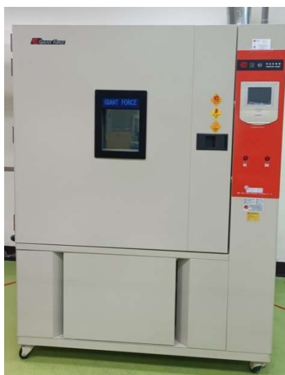
Source: Photo Taken by TPRI Figure 2 Ambient Air Temperature Test equipment
