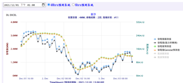
Figure 3 - 6/48 hour wind power forecast for Jinsha Wind Farm
