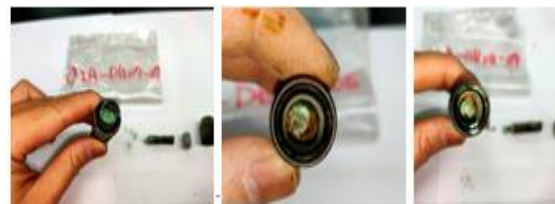
Source: Pictured by TPRI Fig 9 Corrosion products and oxides on the connectors
