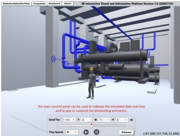
Figure 4 The screen of the front-end 3D platform
