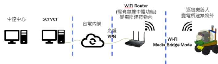
Figure 3 WiFi network architecture diagram
