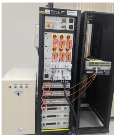
Source: Made by authors Figure. 3 Two virtual synchronous generators operating in parallel: (a)framework, (b)output voltage, current, and power waveforms, (c)physical OPAL-RT system
