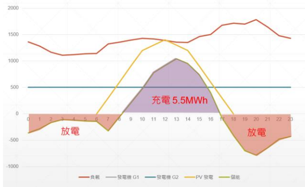
Figure 1 2MW solar energy to be shifted
