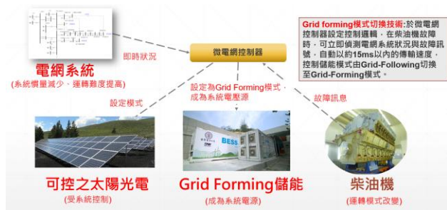
Figure 2 Green Island Power Grid Operation Structure
