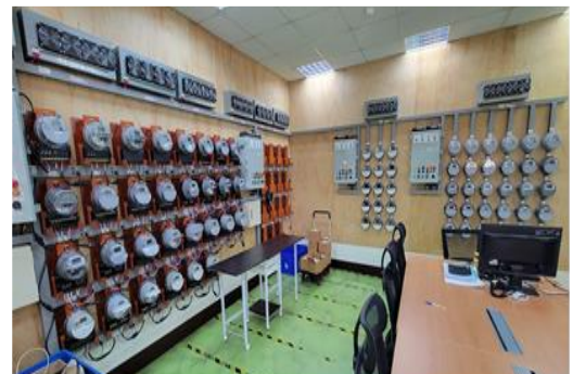
電表與通訊模組交互可用性測試 Operability Testing between Electric Meters and Communication Modules
