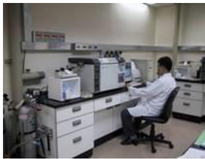
變壓器油中氣體分析 Dissolved Gas Analysis of Transformer Oil
