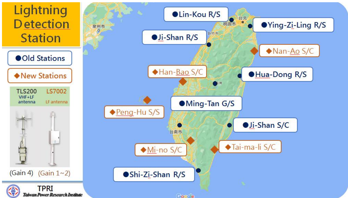
Fig.1 Distribution map of TLS200 and LS7002 lightning detection stations of TPC
