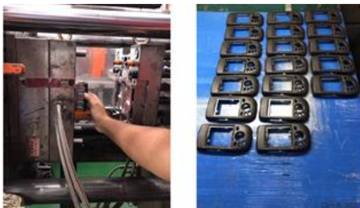
Fig. 3. Composite material granules are manufactured by injection molding machine (left) to manufacture navigation machine shell products (right).
