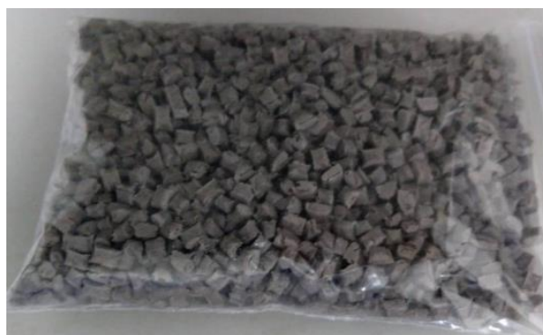
Fig. 2 After the filter bag fragments are unchained, 40% glass fiber is added to the pellets, and the composite material colloids are obtained by twin-screw extrusion.
