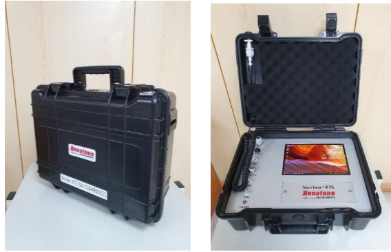
Fig. 3 Design of the portable device for wind turbine blade damage detection
