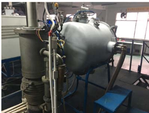
Fig. 1 Schematic Diagram of Vacuum Melting Furnace
